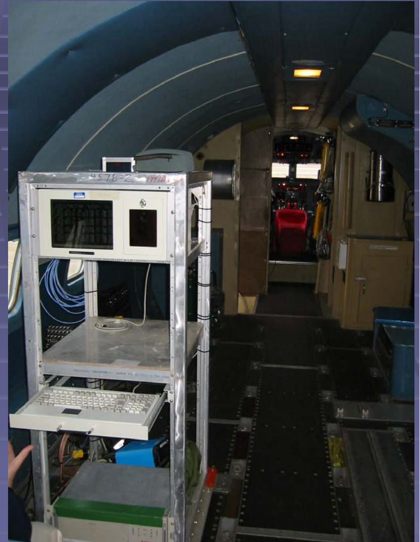
Interior of Convair looking forward; CGA DDC receiver in rack.
